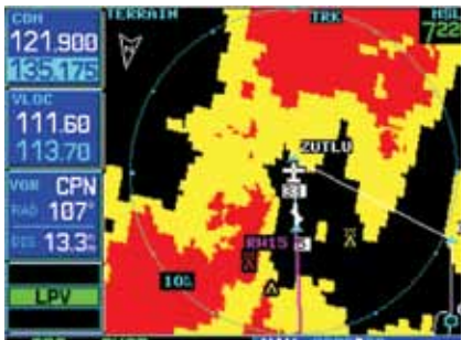
Built-in terrain elevation database can be augmented with optional Class B TAWS alerting capability on the GNS 530W.
