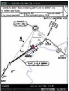
G600: Optional ChartView™ provides a geo-referenced overlay of aircraft position on Jeppesen-format electronic approach charts.
