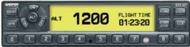
GTX 327 Mode C digital transponder (shown with reversed display)
