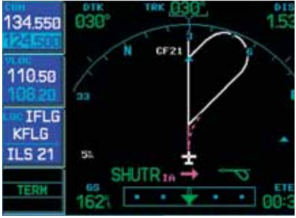
With autopilot-coupled roll steering, both the GNS 430W and 530W can automatically fly the aircraft through holding patterns, procedure turns and other position-critical IFR flight procedures.
