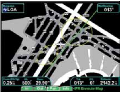
GMX 200: Electronic display of Garmin SafeTaxi® airport diagrams seamlessly depict the current aircraft position in relation to runways, taxiways, hangars, etc.
