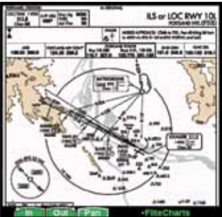
GMX 200: The Garmin FliteCharts® database provides over 14,000 NACO-format approach plates for over 2,900 U.S. airports. FliteCharts® are not geo-referenced (no aircraft position overlaid on chart).
